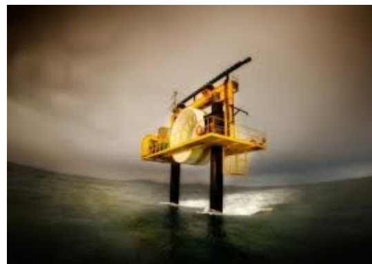
Figure 8: Open Centre Turbine deployed at EMEC
