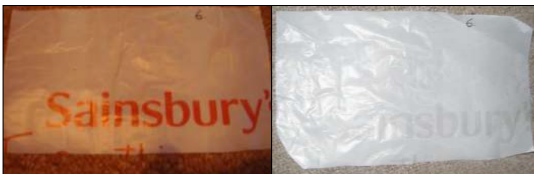
Fig 2.20 Sainsbury samples before and after degradation in salt water
