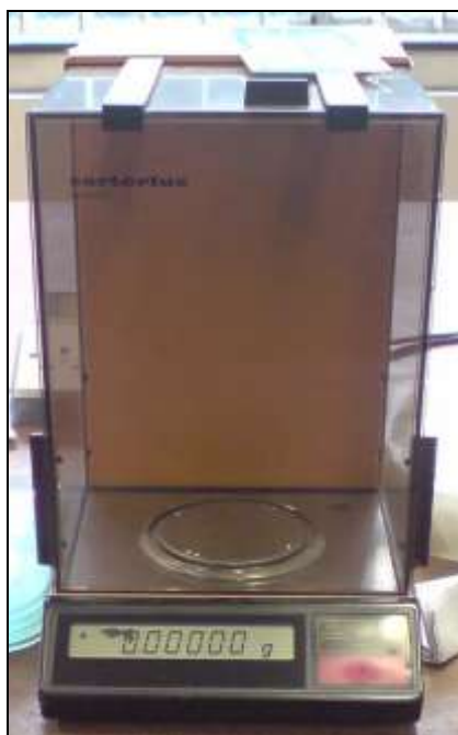
Fig 1.5 Sartorius R200D scales for dry weight comparison
