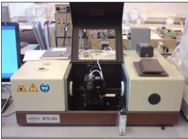
Fig 1.8 Bruker IFS 66 Photo-acoustic device
