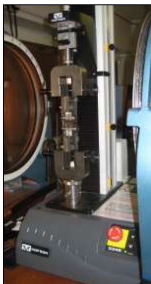
Fig 1.7 Instron 3345 device used for tensile strength recording
