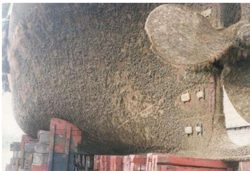
Plate 1. The hull of a ship is prone to fouling organisms. Paint and hull cleaning help decrease the spread of species; however it does not target all areas of a ship and some species are extremely persistent (Geocities 2006).
