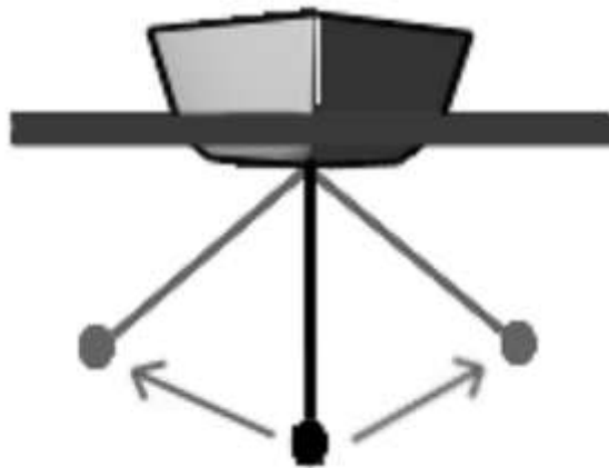
Figure 6. Canting keel concept visualisation, adapted from Canting Ballast Twin Foil Technology
