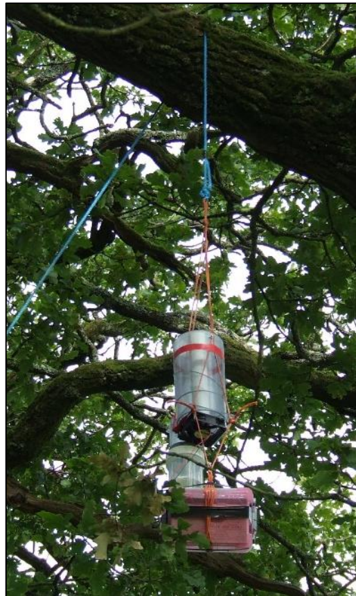
Figure 1: Photograph of fan trap installed in oak canopy (Burchett, n.d.)
