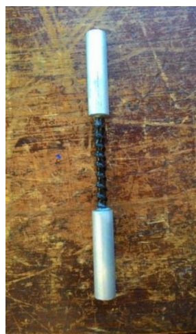
Photo 1: BFRP rebar encased in threaded aluminium rods.
