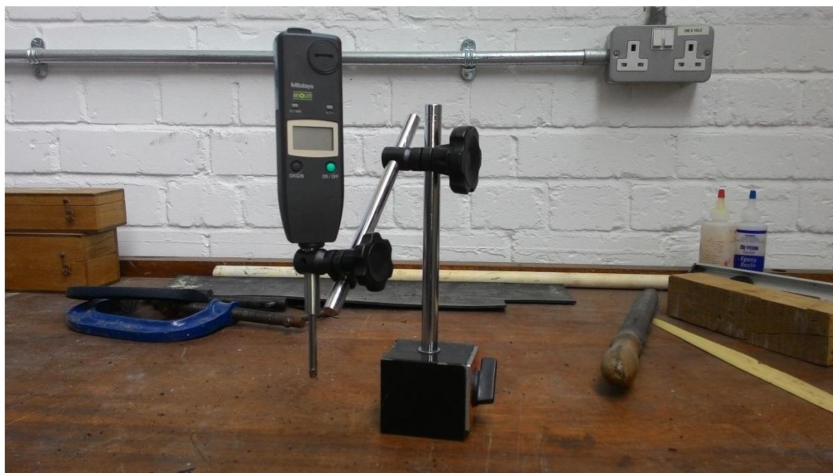
Photo 6: External Vertical Displacement Gauge.
