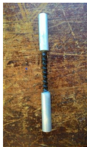
Photo 1: BFRP rebar encased in threaded aluminium rods.
