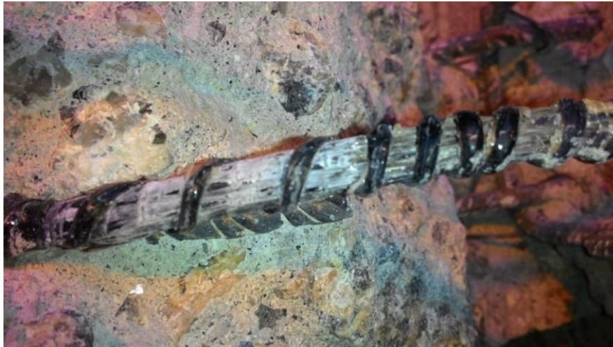
Photo 8: Basalt B2: basalt spiral strands are deboning from longitudinal strands.
