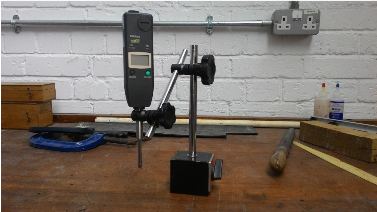
Photo 6: External Vertical Displacement Gauge.
