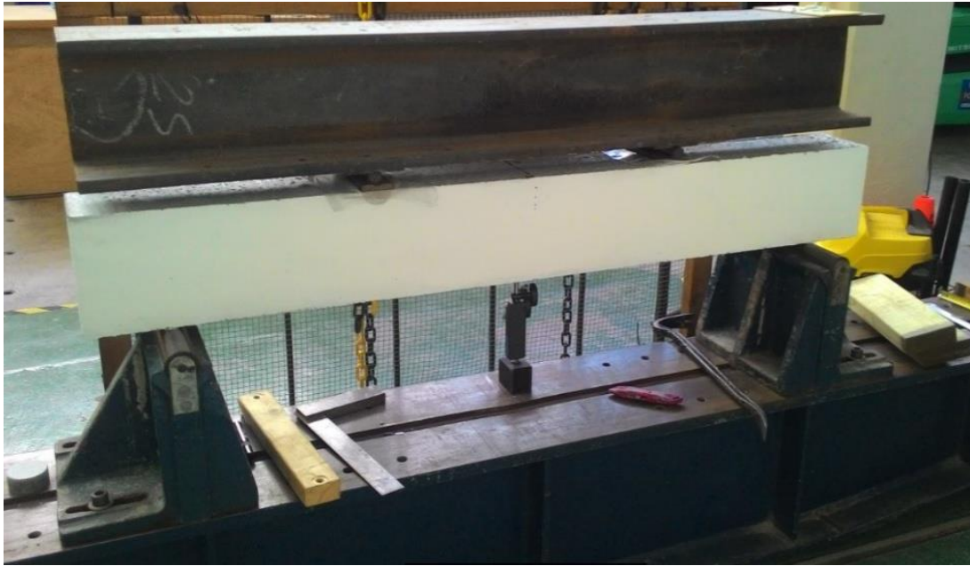
Photo 5: R.C. Beam Two-Point Load Setup.
