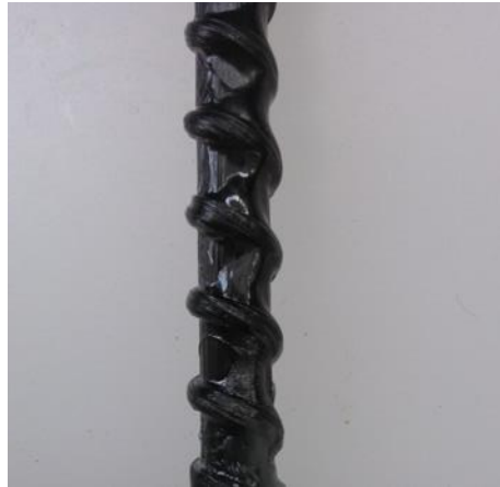
Figure 1: Basalt Fibre Reinforced Polymer rebar.
