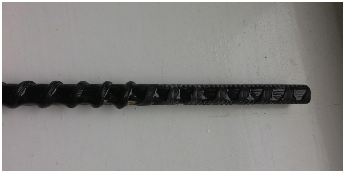
Photo 2: Ends of BFRP Rebar Sanded Off.
