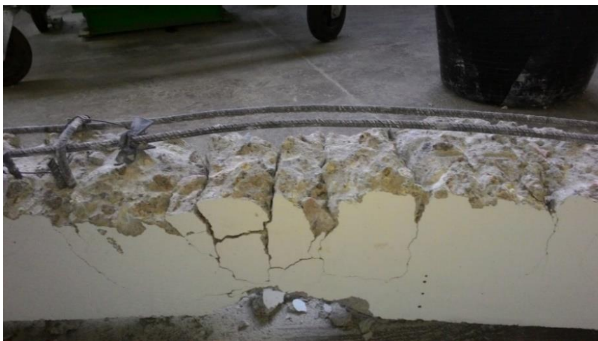
Photo 7: Beam B1 Yielded Tension Steel Bars.
