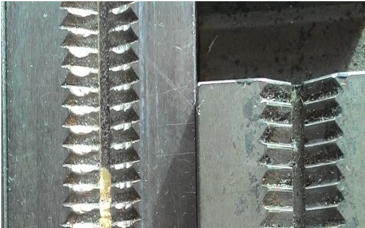
Photo 5 – Damaged Upper Tensile Strength Testing Machine Clamp.
