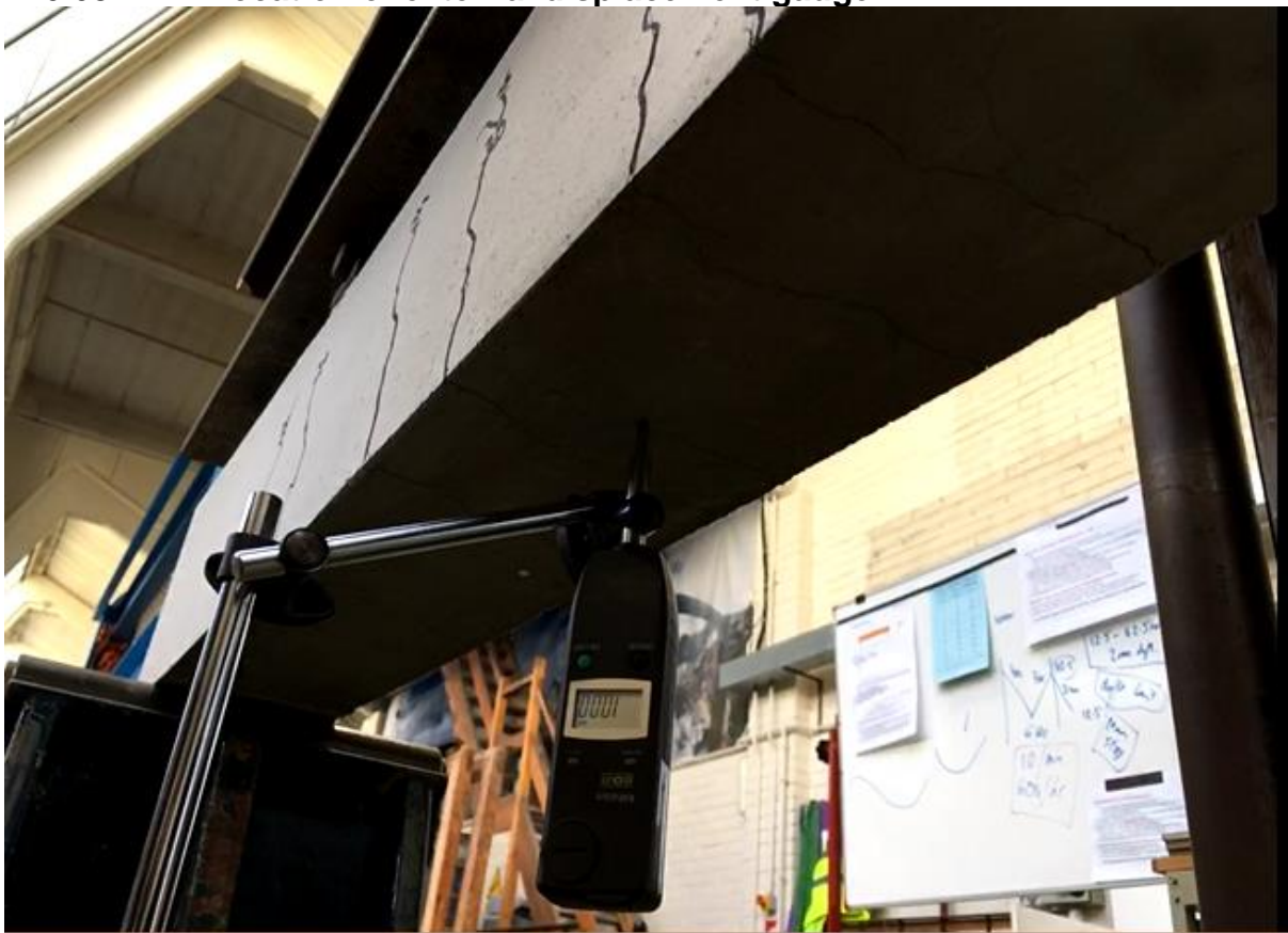
Photo 11 – External Vertical Displacement Gauge Location 1.
