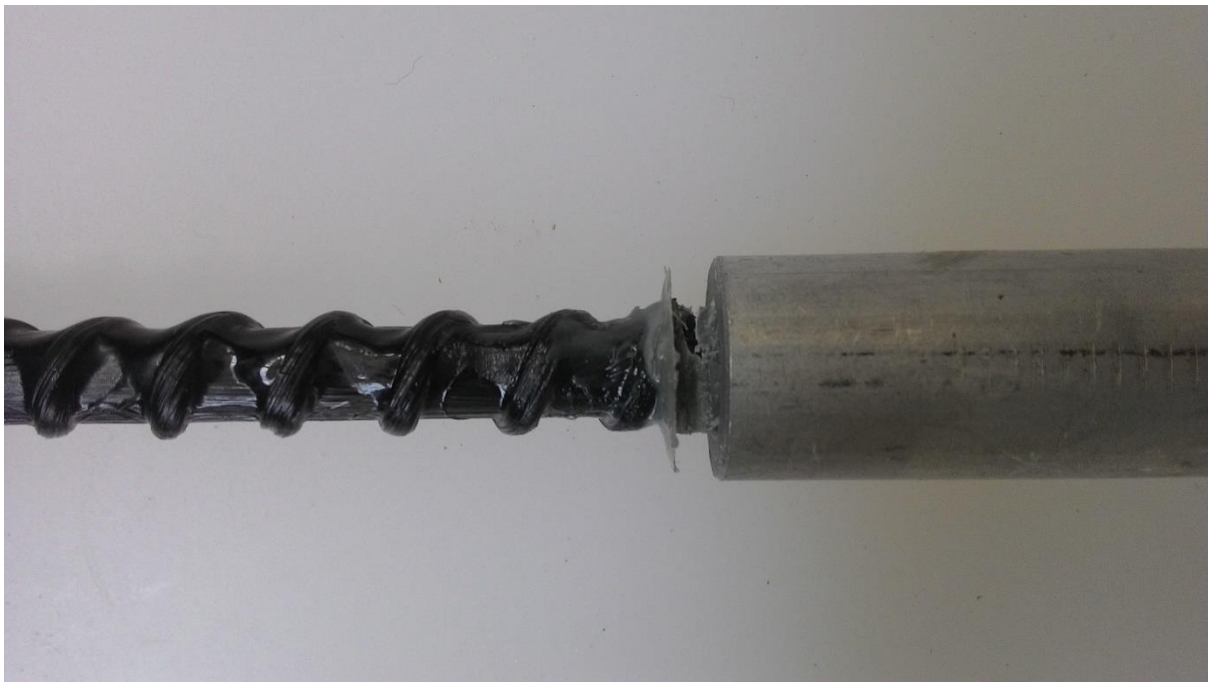
Photo 2 – BFRP Rebar Pulled Out from Aluminium Encasement.
