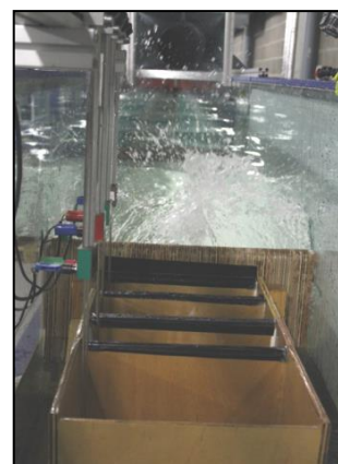
Figure 12: Wind causing splash overtopping into the first collection bucket
