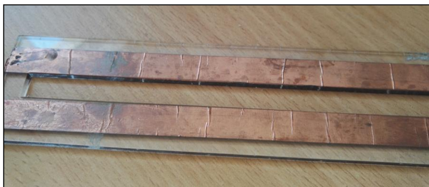
Figure 41: Potential oxidation to the wave gauges
