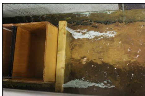
Figure 39: Water escaping the collection buckets at the higher wind speeds
