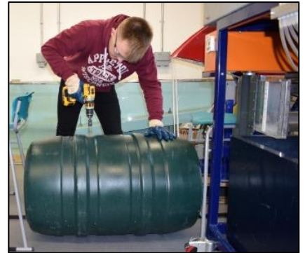
Figure 29: Drilling holes for pipe attachments
