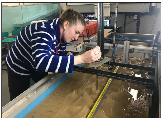
Figure 6: Using the shadows produced by the vertical sand level gauge to ensure the measurement is being taken on the surface of the sediment
