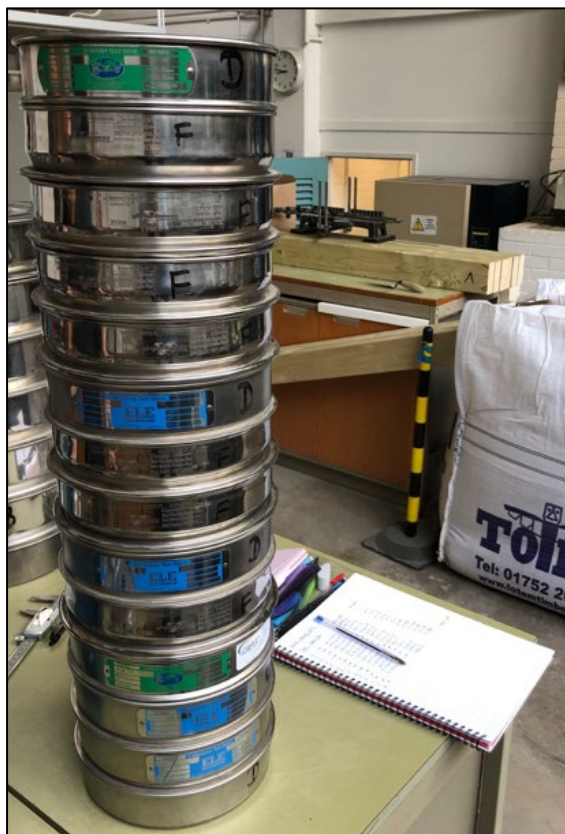
Figure 6: Sieve stack for gradation – 10 sieves with decreasing mesh sizes
