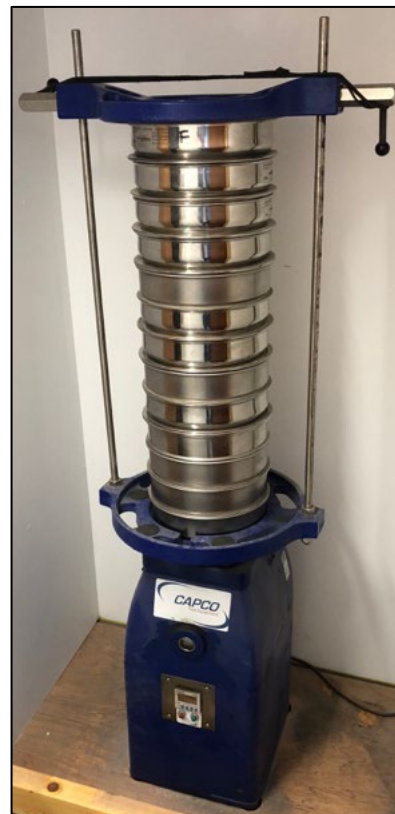
Figure 7: Shaker used to ensure sample separated entirely into the correct sieves
