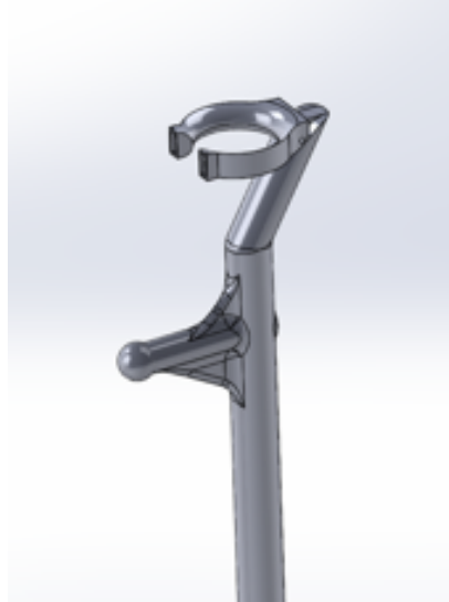
Figure 24: Shows a possible design for a composite tubing design manufactured from 2 composite tubes with either sleeve hand grip or (as shown) a integrated handle design. These ideas would produce very lightweight composite crutches, with the bought in tubing design being very cost affective.
