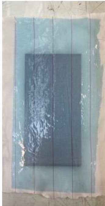
Figure 32: the pre-preg plate, pre-cure, pre-bagging and autoclave process. The sample material was provided by SHD Composites, 3 x 400mm x 400mm sheets of MTC400-1-C200T-HS-3K-42%RW-1250.
