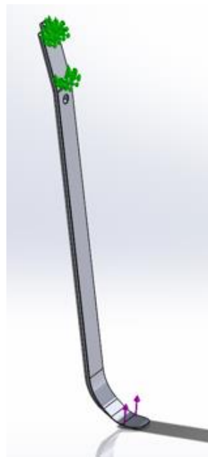
Figure 37: Image of CAD Crutch with loading points at the bottom and fixed at the top, the top being fixed at the whole of the top face due to that being between the two places the athlete interacts with the crutch making deformation there very unlikely due to the strength of that area. The Load (1000N) was applied as during in testing the biggest stress was roughly 40kg so a safety factor of 2.5 could be seen if the crutch could withstand this load.
