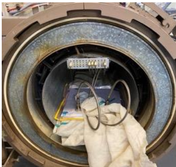
Figure 34: composite plate on fully pre-prepared glass plate, enveloped bag with valves attached to the pipes in the autoclave and temperature sensor on the component to ensure there is no leakage in the bag and the plate is at the temperature specified.
