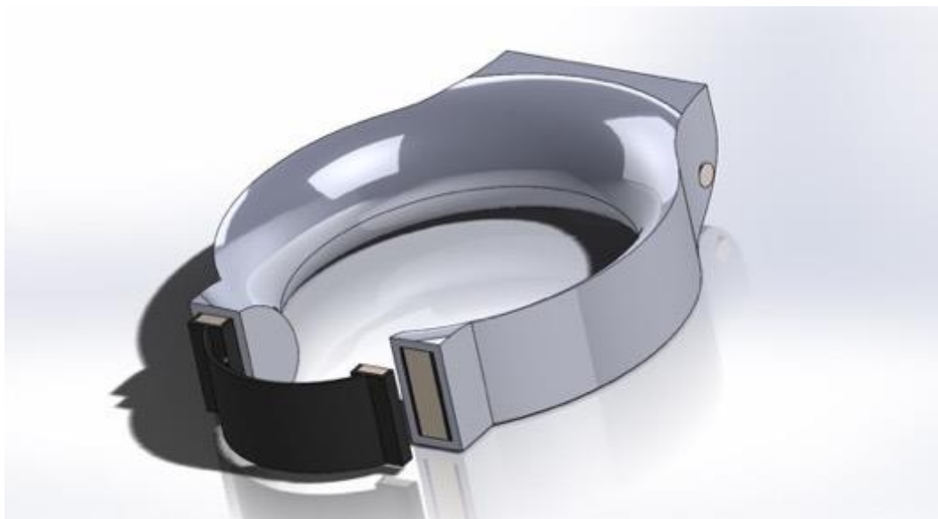
Figure 27: Shows the Arm Supports system with its magnetic release strap. The system consists of two magnets that are enclosed in the arm support (cuff) and an elastic strap attached with 2 magnets. When closed it will be strong enough to hold the weight of the crutch on the athletes arm but also allow the athletes arm to remove from the cuff at any point.
