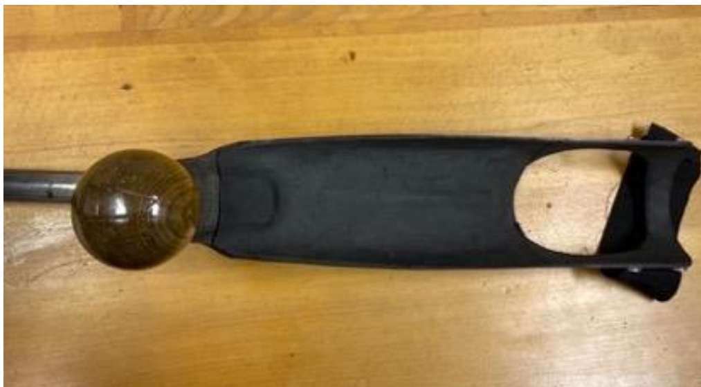
Figure 3: Compared to the current crutch, majority of the force is distributed through the forearm but due to the composite crutches forearm support being just an elastic strap all forces are distributed to the hand and underarm which is not practical.
