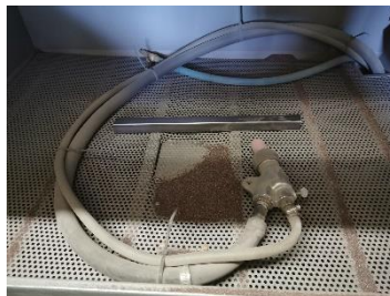
Figure 11: Tube Cut Length in Blasting Cabinet
