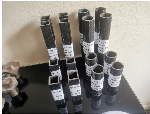
Figure 18: Composite Clad Specimen Samples Weighed and Labelled
