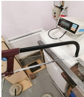
Figure 7: Cutting Steel Stock to Length
