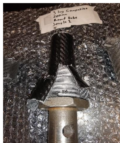
Figure 27: Local Buckling of 200mm Reinforced Specimen 3LC200R1
