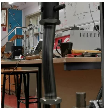
Figure 26: Global Buckling of 200mm Specimen P200R1
