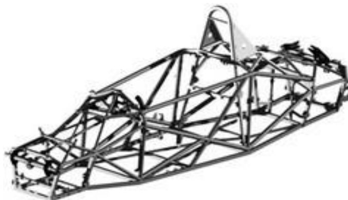
Figure 1: Space Frame Chassis with permission (Clarke, 2009)
