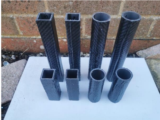
Figure 17: Composite Clad Steel Tubes Cut to Length
