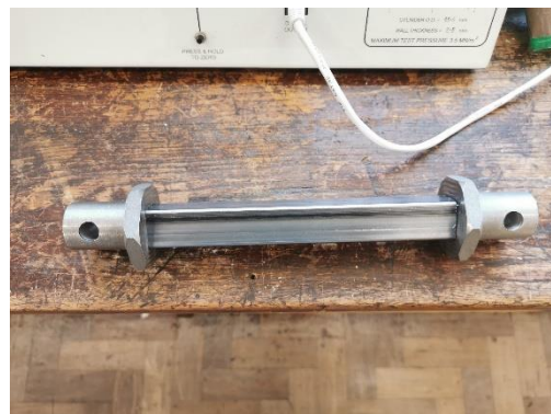
Figure 20: Adapters Fitted to Specimen
