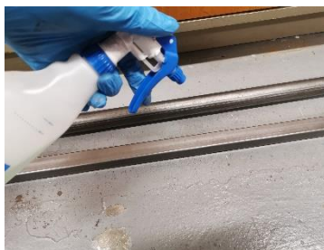
Figure 10: Degreasing Steel Stock
