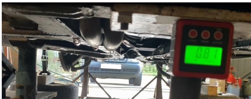
Figure 24: Position 11 twist measured directly off fixture plate
