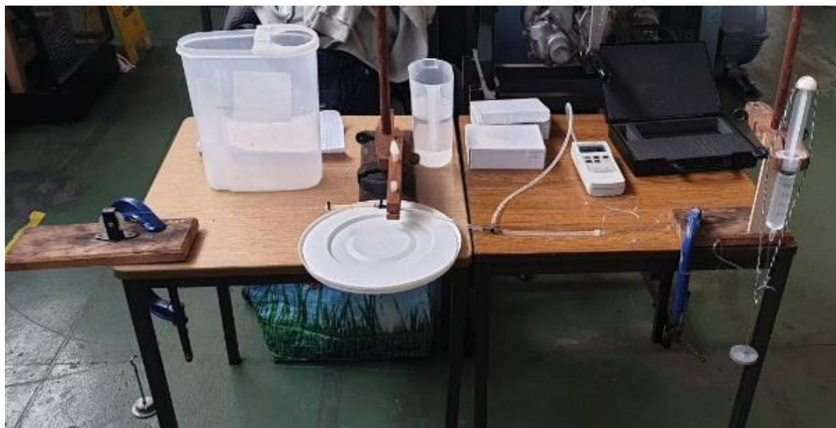
Figure 11: Rig set up for CT method. Prior to 3-way valve addition which was added to refill the syringe
