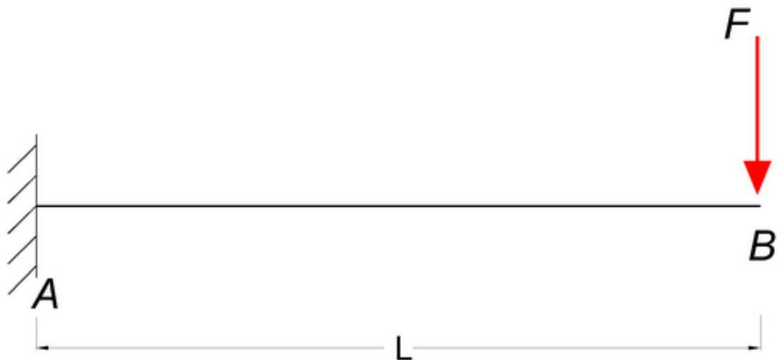
Figure 36: Cantilever beam schematic, point load
