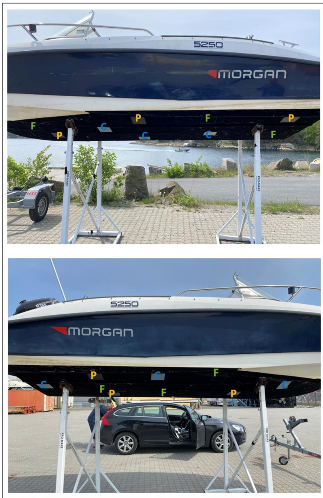
Figure 3: Plastic pleasure boat used for boat hull survey with six quadrats for each treatment: C= control, P= paint, and F= fibre.
