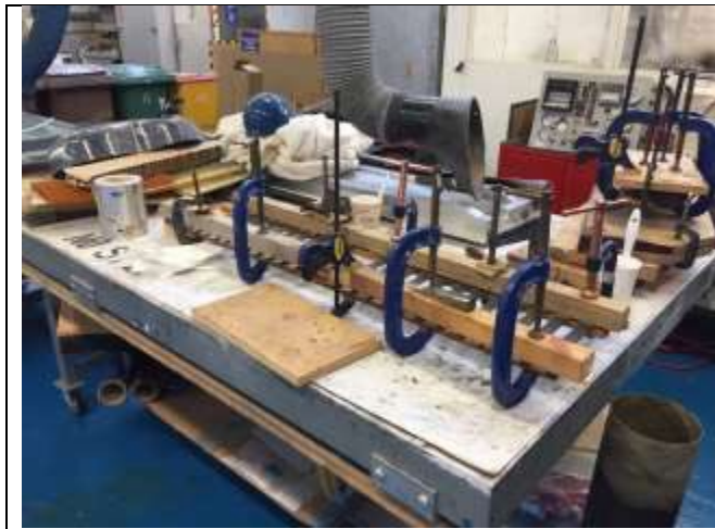
27. Glass fibre tabs are then bonded and clamped.
