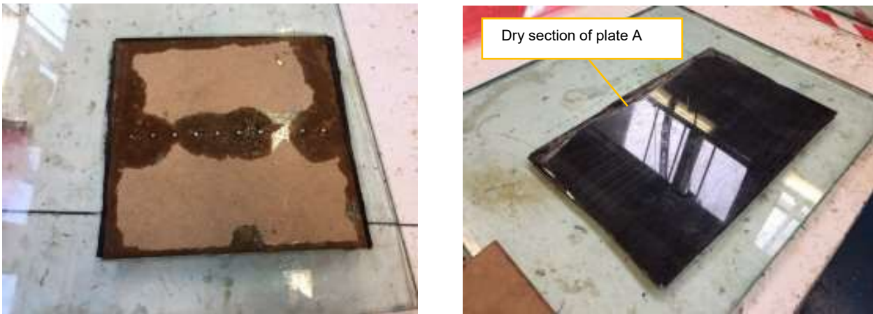
Figure 21: Left: resin seep around the mould tool, right: mirror like surface of plate A.
