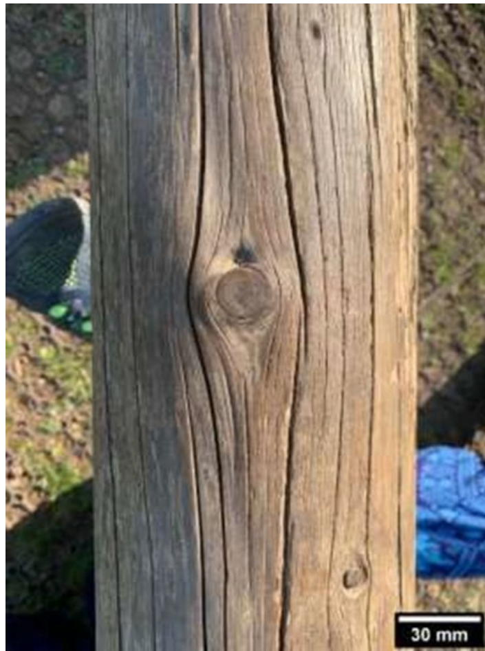
Figure 4: Example tree knots showing curvilinear fibre path.
