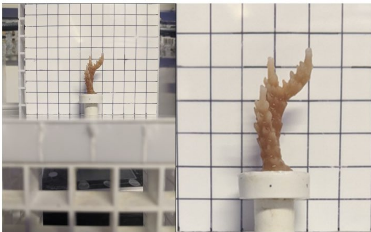
Figure 3: Photograph collection using a 1cm x 1cm square grid stand, to retrieve longitudinal photographic data of coral pigmentation. Using reference centre alignments, the camera was centred to the base of the stand and images were cropped to reveal the final raw JPG File image.
