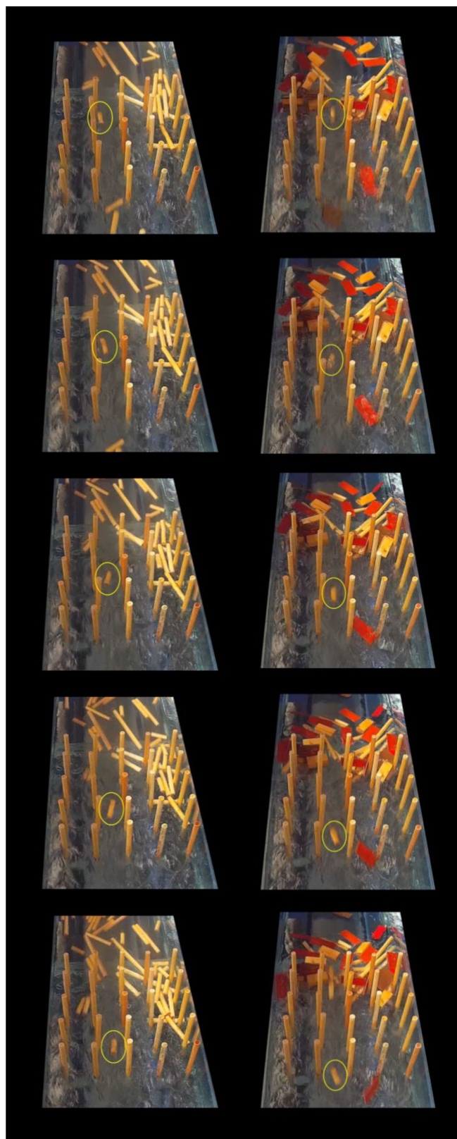
FIGURE 11 Video frames selected at 1/6 s intervals to track the motion of a small cylinder through obstacle array: LHS (no dam) and RHS (with dam).
