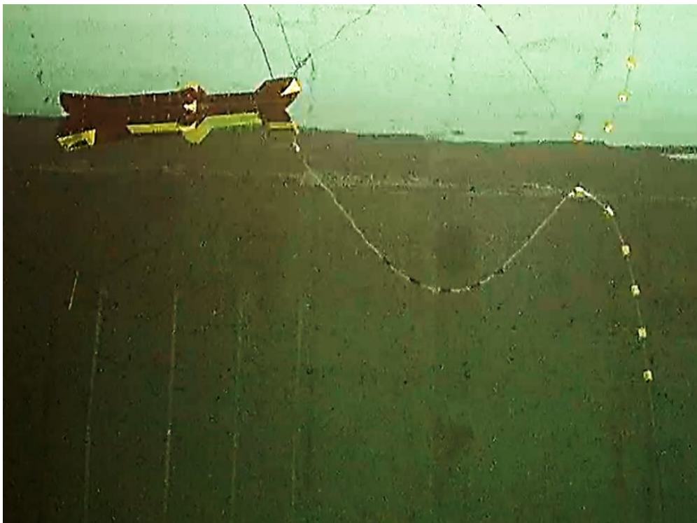
Figure 4.1: Subsurface view of model WEC and Lazy S mooring line - experimental setup
