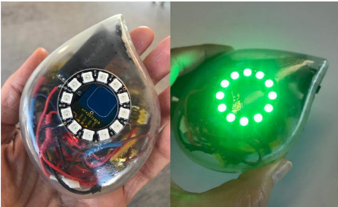
Figure 5.7: Clear/transparent resin for 3D printed casing (Hurban, 2021)
