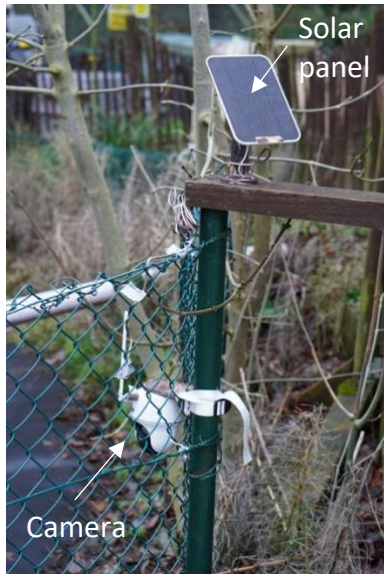
Figure S1 (left): Reolink Go PT Plus (Reolink, China) in Nursery pool (camera 2). Camera is attached to the pole using supplied strap. Solar panel charges the camera and is placed in a place that will get direct sunlight to be able to charge the cameras.
